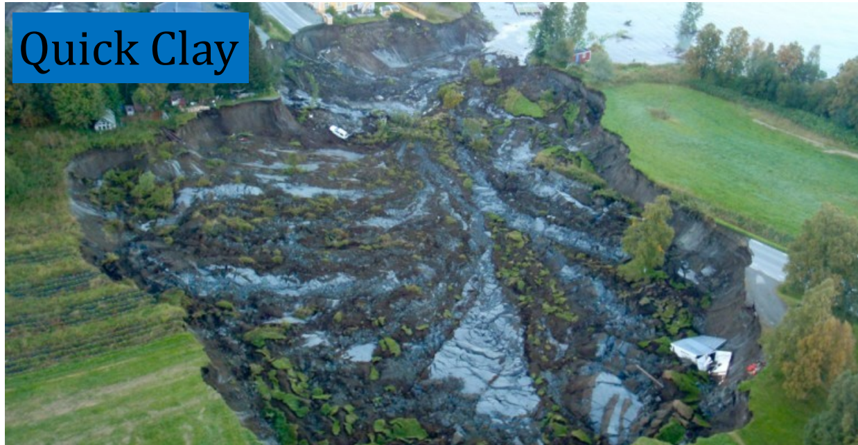
Picture: Quick clay landslide at Lyngseidet, September 3, 2010 (220.000 m 3 ). The landslide was likely triggered by loading of fill along the shoreline. Photo: Andrea Taurisano, NVE
